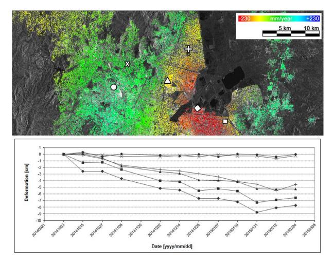
Figure 3. Deformation map (top) of the processed burst encompassing a large area of Mexico
