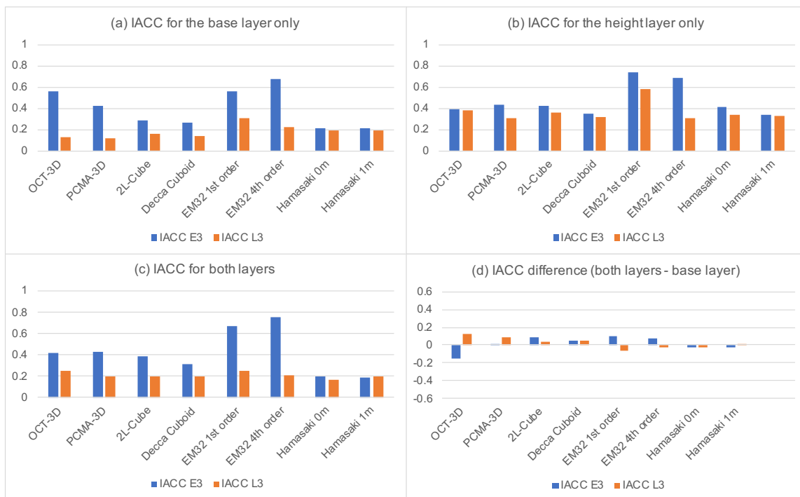
Fig. 8. Interaural cross-correlation coefficients (IACCs) for ear-input signals resulting from different microphone signals reproduced from a binaurally synthesised 9-channel 3D loudspeaker system.
