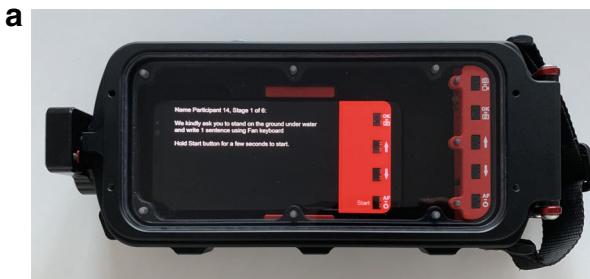
a Samsung S8 sealed in Diveshot, a waterproof housing from Easydive. The smartphone cannot be accessed directly by divers and is controlled by five optical buttons in the right part of the housing. The participants operate the lower four buttons that correspond to the four buttons of the application. The fifth, top-most button is used by the supervisor to access and change the experiment's settings.
