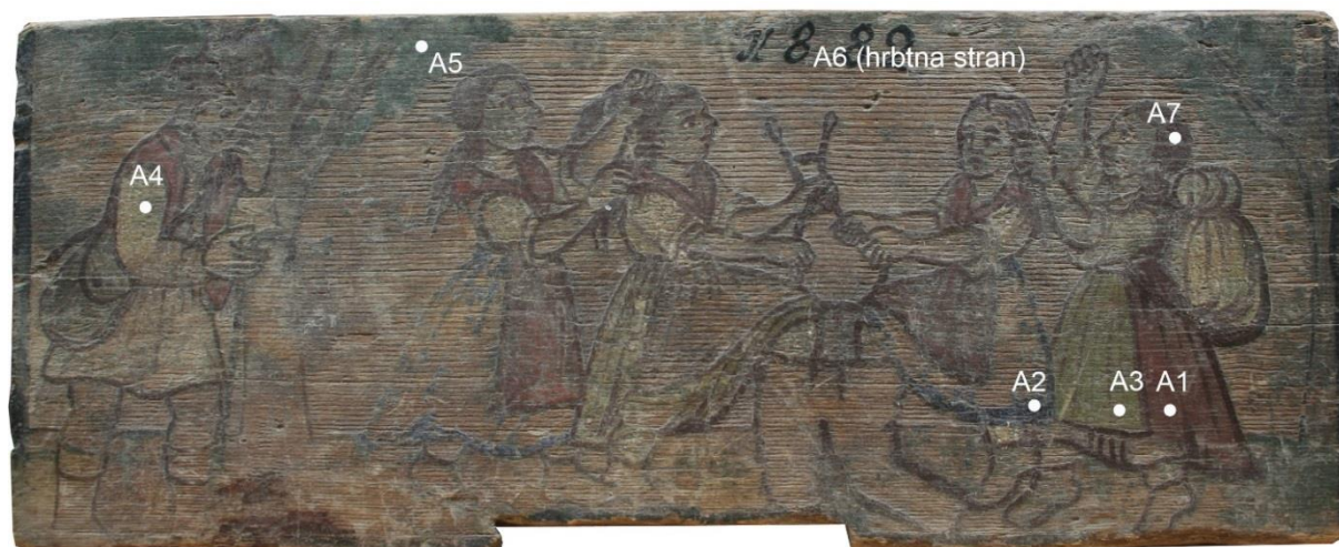
Figure 11: Marked locations of reflection FTIR analysis.
