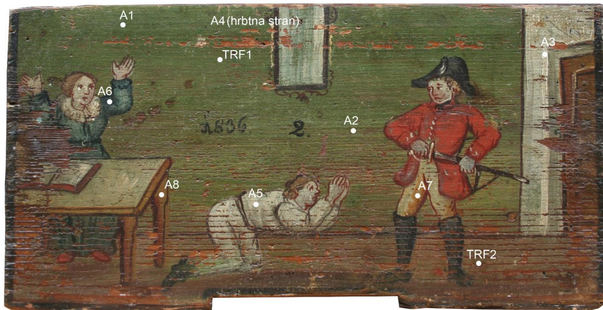
Figure 3: Marked locations of reflection and transreflection FTIR analysis.
