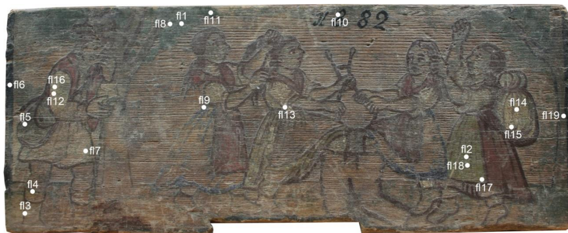
Figure 21: Locations of noninvasive Raman measurements of beehive panel marked as PK2, where material identification was not possible due to fluorescence
