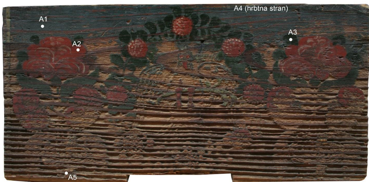
Figure 23: Marked locations of reflection FTIR analysis.
