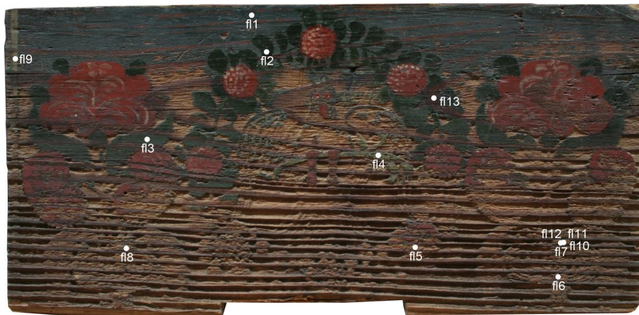
Figure 27: Locations of noninvasive Raman measurements of beehive panel marked as PK3, where material identification was not possible due to fluorescence
