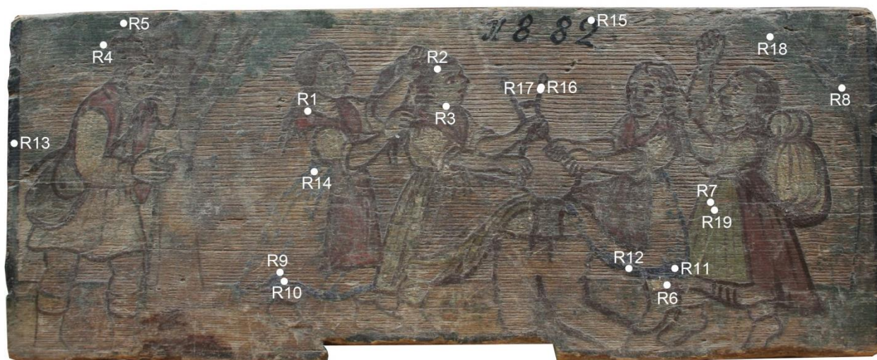
Figure 10: Marked locations of Raman analysis.
