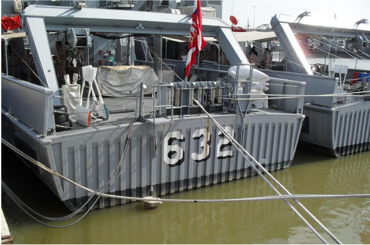
Figure 2. Wooden hulls on stainless steel frames, with vessels in the water for over 30 years hull repairs would be necessary, using skills which were fast becoming difficult to find
