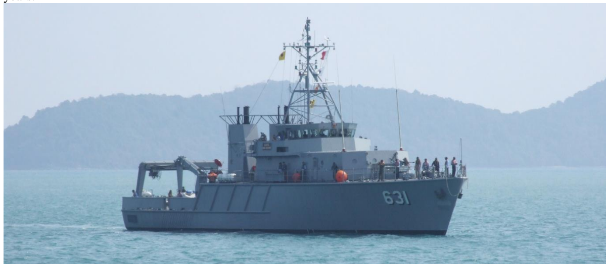
Figure 1. Bang Rachan Class MCM: 48m LOA at 450 Tonnes displacement
