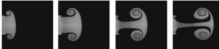
Figure 4.5.: Vortex ring formation in the wake of a starting jet from Olcay and Krueger (2008).
