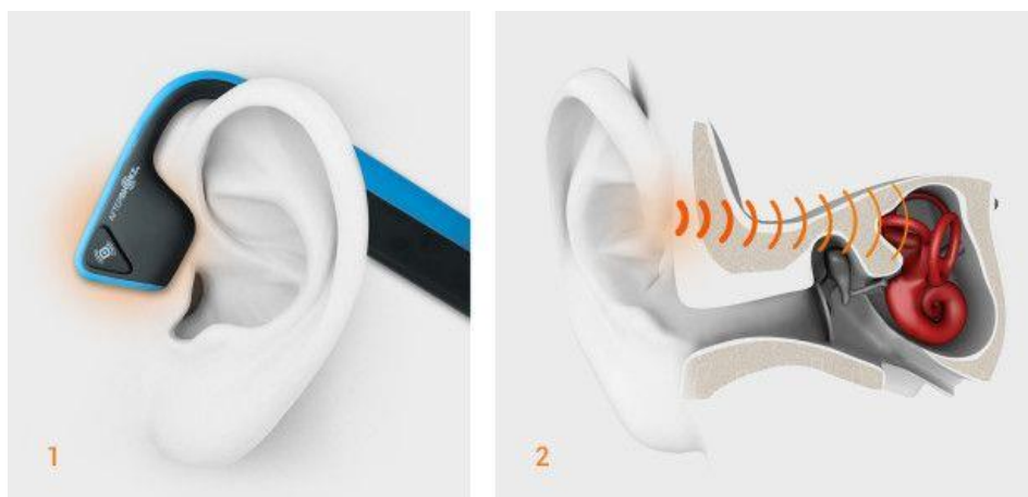
Figure 5 : illustration of the two types of listening (classic and bone conduction)
