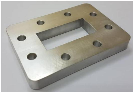
Figure 1. Mold for casting cement-graphite block
