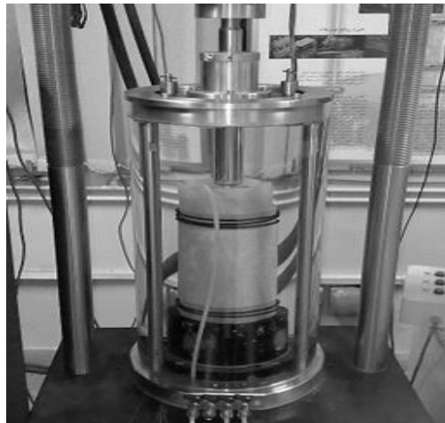
Figure 2 Plastic concrete specimen during testing
