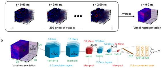
Figure 1: General workflow for using classical molecular dynamics simulations and 3D convolutional neural networks to make predictions of experimental kinetic solvent parameters ( $\sigma$ ). (a) Conversion of MD configurations into voxel representations. (b) SolventNet architecture that interprets voxel representations and outputs  $\sigma$ . Additional details can be found in the main text.
