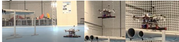
Figure 17. MHYRO landing in a pipe rack
