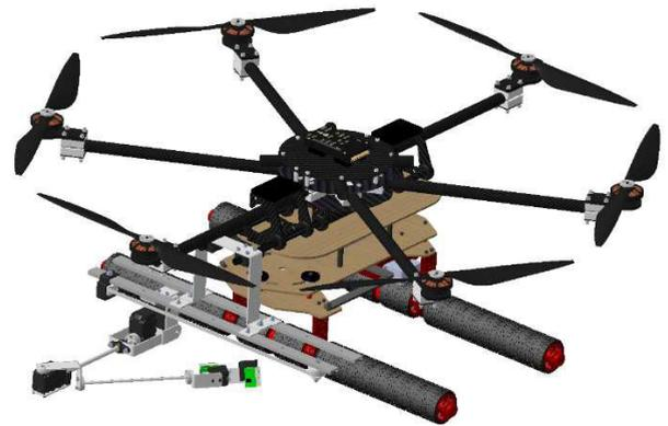
**FIGURE 4. Rendered view of the rolling-aerial manipulator.**
