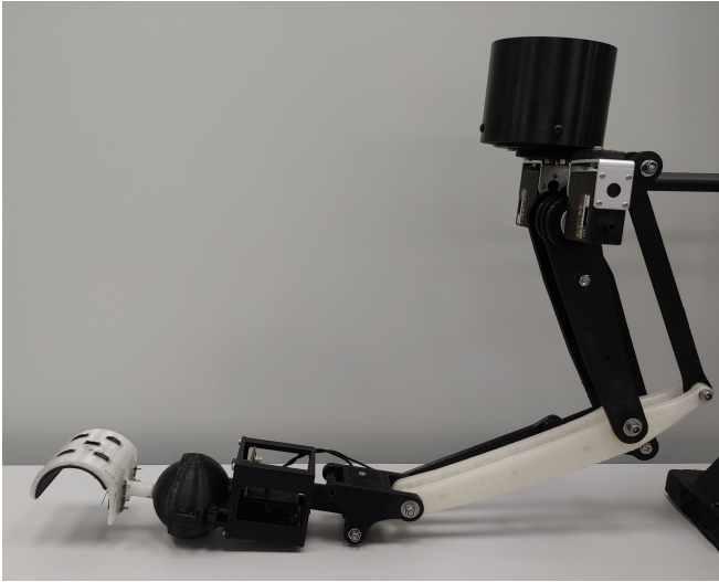
Fig. 6. Real implementation of the robotic arm with the positioner tool.
