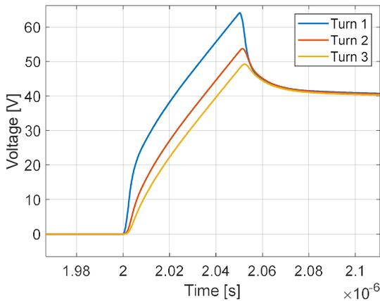
Fig. 11 Voltage drop across 1<sup>st</sup>, 2<sup>nd</sup> and 3<sup>rd</sup> turns.
