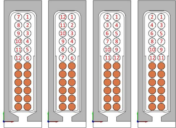
Fig. 8 Example of 4 configurations with different conductors' location.
