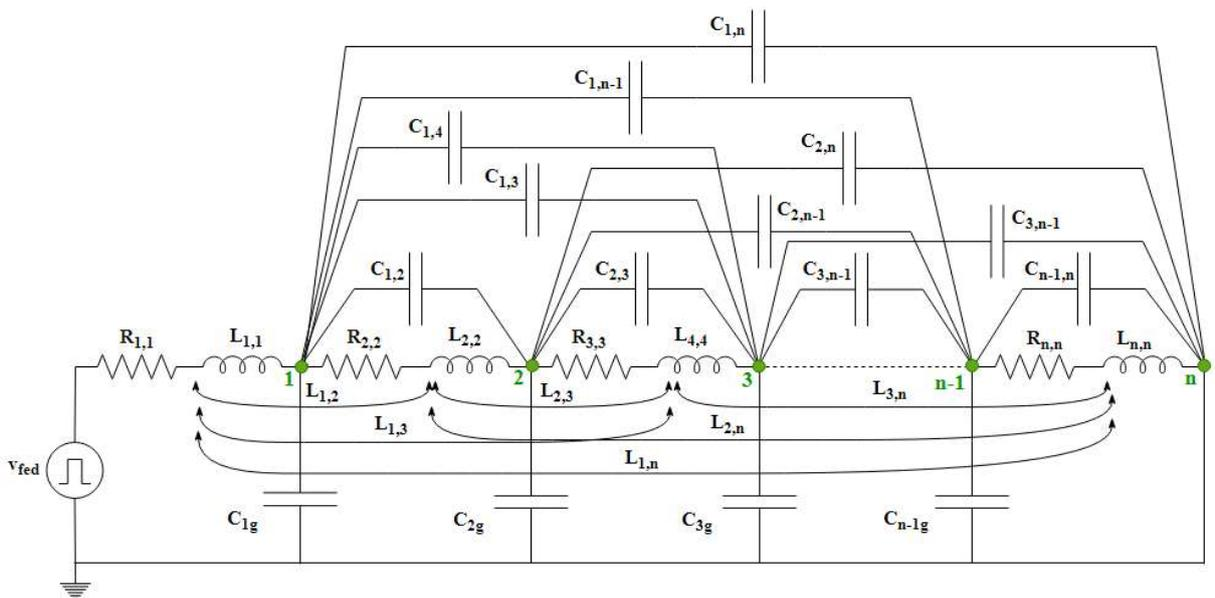
Fig. 1 Equivalent circuit of a winding coil
