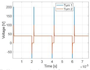
Fig. 5 Instantaneous voltage drop across the first two turns (Turn 1 and Turn 2). Duty cycle 90%.
