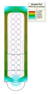
Fig. 3 2D FE model of the slot: flux lines are mainly confined in the ferromagnetic part outside the slot.
