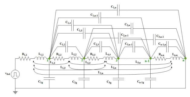
Fig. 1 Equivalent circuit of a winding coil
