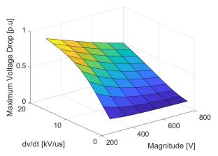
Fig. 7 3D map of the instantaneous maximum voltage drop across the first turn in p.u.  $% \left( {{{\mathbf{x}}_{i}}} \right)$
