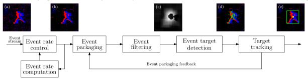
Fig. 2: Event-based target detection and tracking scheme: a) event stream representation, b) event stream representation after random discard procedure, c) APM obtained for event filtering, d) corner tracking, e) event clustering and, f) target tracking.
