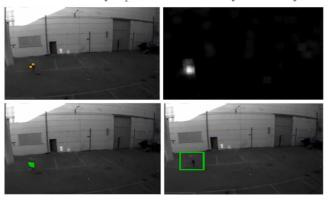
Fig. 6: Results of day experiments: top) events over framebased images (left) and resulting APM (right); bottom) result of target detection (left) and tracking (right).
