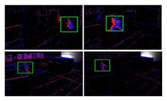
Fig. 7: Detection and tracking results in dark (top) and dynamic (bottom) lighting conditions experiments.
