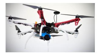
Fig. 5: Robot used in the shown experiments: a DJI Flamewheel F550 platform with a DAVIS 346 and an INTEL NUC.
