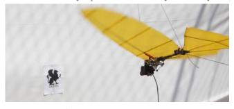
Fig. 3: Set-up of the motion-blur experiment with a DAVIS 346 sensor onboard a flapping-wing ornithopter.
