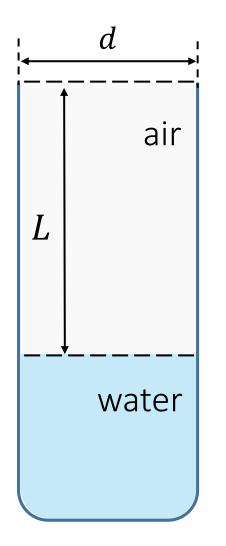
c – speed of sound in the air 0.2d – end correction
