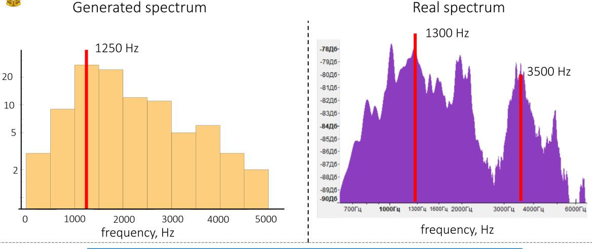
Spectrum is partially continuous  $\rightarrow$  sound is produced by bubbles
