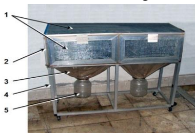
Figure (1): Two of the cages used for the mass rearing of Sitotroga cerealella . 1. Steel mesh, 2. Upper part of the cage, 3. Funnel, 4. Metal stand and 5. Collecting plastic jar.
