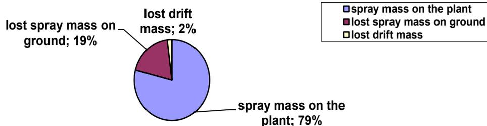
Figure (15b): Distribution of spray mass on the plant, lost on ground and the drift spray for knapsack motor sprayer Agrimondo with charging unit (42) L / fed.
