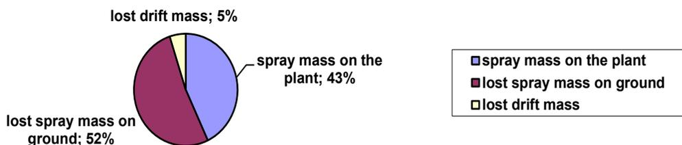
Figure (15a): Distribution of spray mass on the plant, lost on ground and the drift spray for rotary matabi sprayer (18) L / fed.
