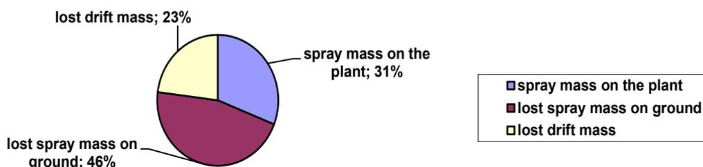
Figure (15c): Distribution of spray mass on the plant, lost on ground and the drift spray for hydraulic matabi sprayers ( 56) L / fed.
