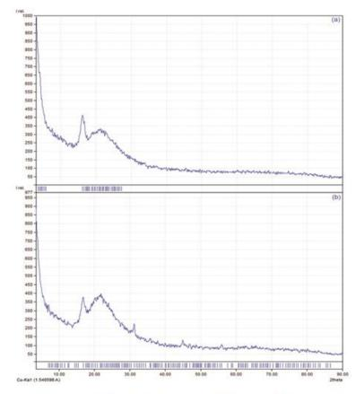
Figure (2): X-ray diffraction pattern graphics of SiO<sub>2</sub> crystals (a) and SiO<sub>2</sub>nanaoparticles (b).
