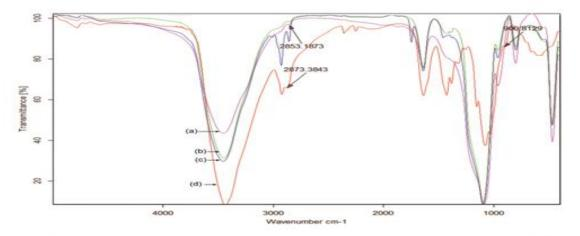
Figur e (4): FTIR spectra of SiO<sub>2</sub> crystals (a), SiO<sub>2</sub> nanaoparticles, NPs (b), SiO<sub>2</sub> nanaopaticles contained clove oil, SLN/clove of peppermint.
