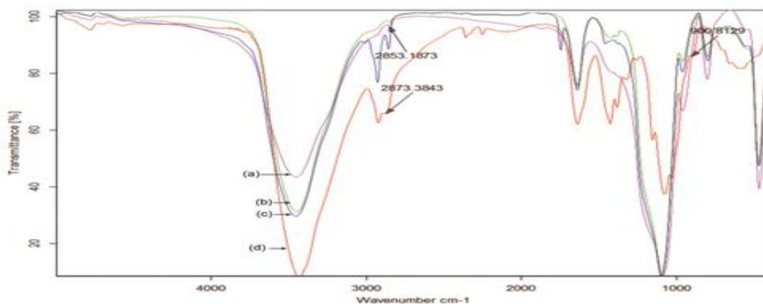
Figure (4): FTIR spectra of SiO<sub>2</sub> crystals (a), SiO<sub>2</sub> nanop articles, NPs (b), SiO<sub>2</sub> nanop articles contained clove oil, SLN/clove of p eppermint.
