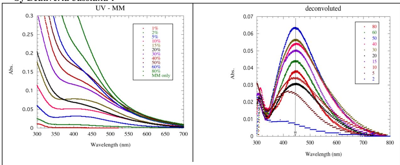
**Figure (3): UV-Vis spectra response of silver nanoparticles by *Metarhizium brunneum* .**
