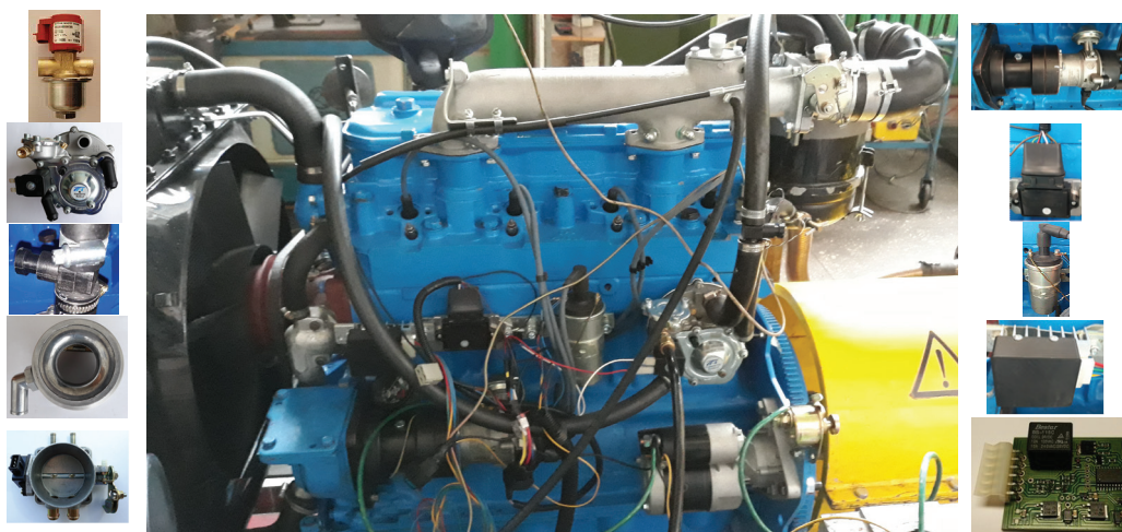
Fig. 1. External view of the D-240-LPG-”A” gas internal combustion engine with the main and additional systems, as well as their elements and the Avenir Gaz 37 “A” ECU
