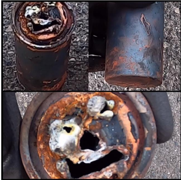
45 46 Fig. S6. Deployed hexachloroethane grenade 6: 17 July 2020, SW 3rd between Madison and Jefferson, 47 detonated, observed deployed, recovered. Photos by the author.
