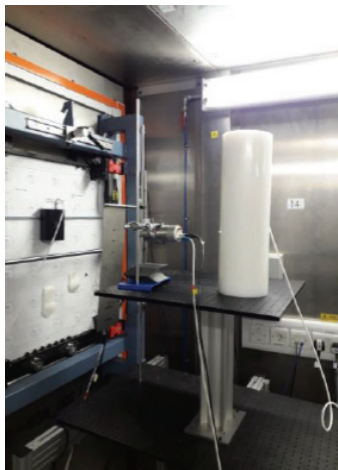
Figure 2 Delayed neutron detectors set up on ChipIR.
