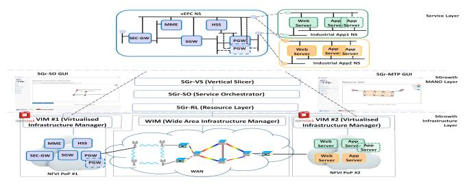
Figure 1: Scaling of composite NSs over the 5Growth platform
