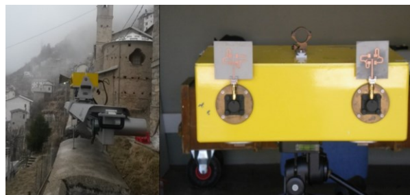
Fig. 1. (Left) Picture of the Radar system installation (VV mode configuration). (Right) Picture of the transceiver mounting the two circularly polarized antennas.
