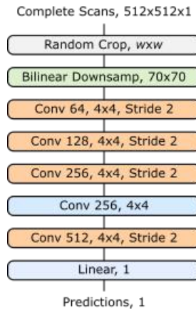
Figure S1. Discriminators examine random w \times w crops to predict whether complete scans are real or generated. Generators are trained by multiple discriminators with different w . This figure was created with Inkscape 1 .
