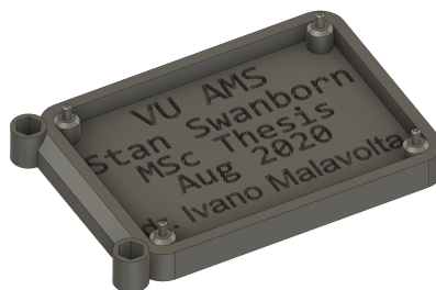
Figure 3.18: The circuit mount as designed and 3D printed.
