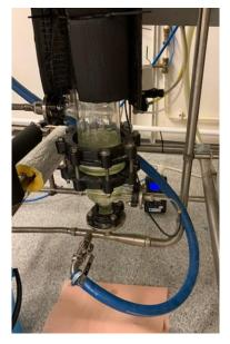
Figure 4 CHE626 automated absorption and stripping pilot plant operating at batch mode (recirculation).
