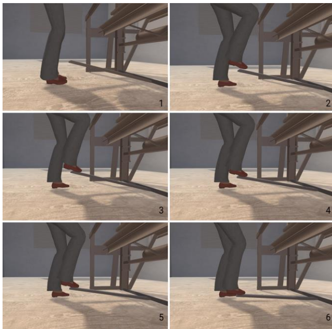
Figure 8. Detail of the foot of the VH operating the treadle while loom weaving.
