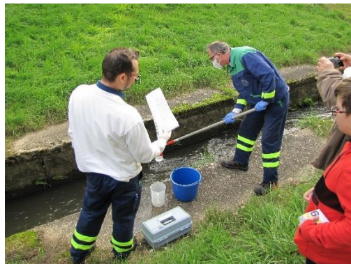
The experts of the Budapest Sewage Works taking their regular, bi-annual water sample for monitoring (Photo: Balázs Kozák)
