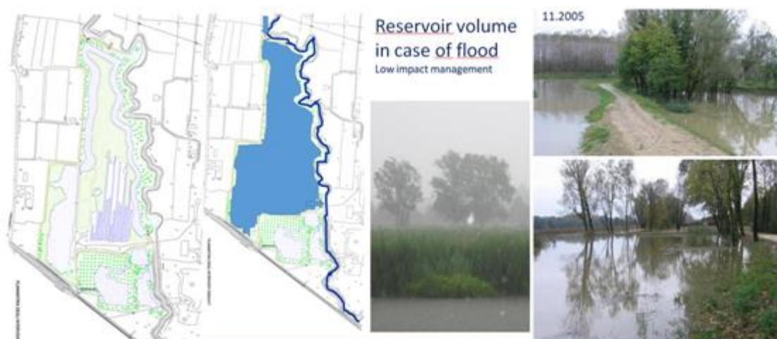
Figure 4: Reservoir area in case of flood with some glimpses of the wetland during a high flood (map and photos of courtesy DA "Acque Risorgive").
