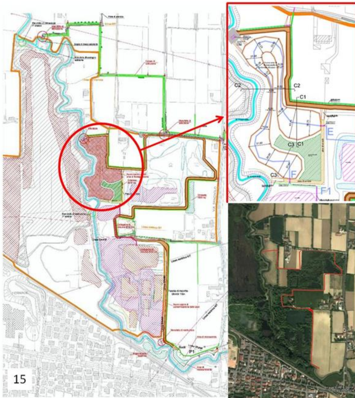
Figure 6: Details of the new restoration project, in particular the transformation from arable field to wetland (map and photos of courtesy DA "Acque Risorgive").
