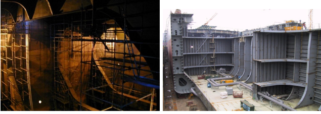
Figure 1: (left) Staging required during a vessel inspection. (right) Oil tanker in shipyard during construction.
