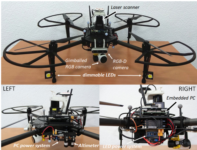
Figure 2: ROBINs aerial platform, fitted with a laser scanner, a height sensor, a camera set featuring LED-based illumination, and an embedded PC.
