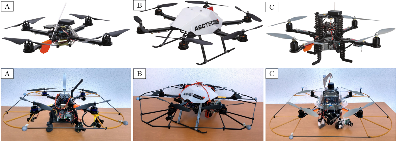
Figure 9: (Top) The aerial platforms as delivered by the manufacturer: (A) Hummingbird, (B) Firefly, and (C) Pelican. (Bottom) the platforms equipped with the sensor suites, on-board computers and cameras.
