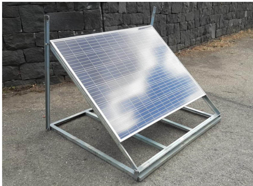
Figure 3 - Foldable galvanized-steel structure holding the solar panel of the MEMS station. The structure allows for different tilt angles of the panel.
