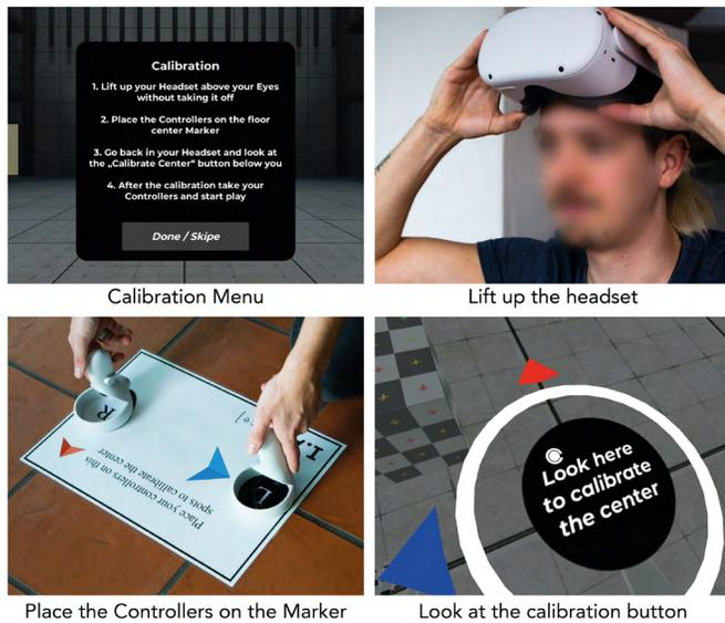
Figure 4: Calibration process Source: Leisi and Sahli
