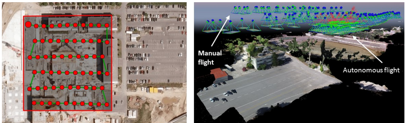
Fig. 4 Trials in Athens (May 2016): area with fly paths (left) and a complete 3D model (right) for Test area #1
