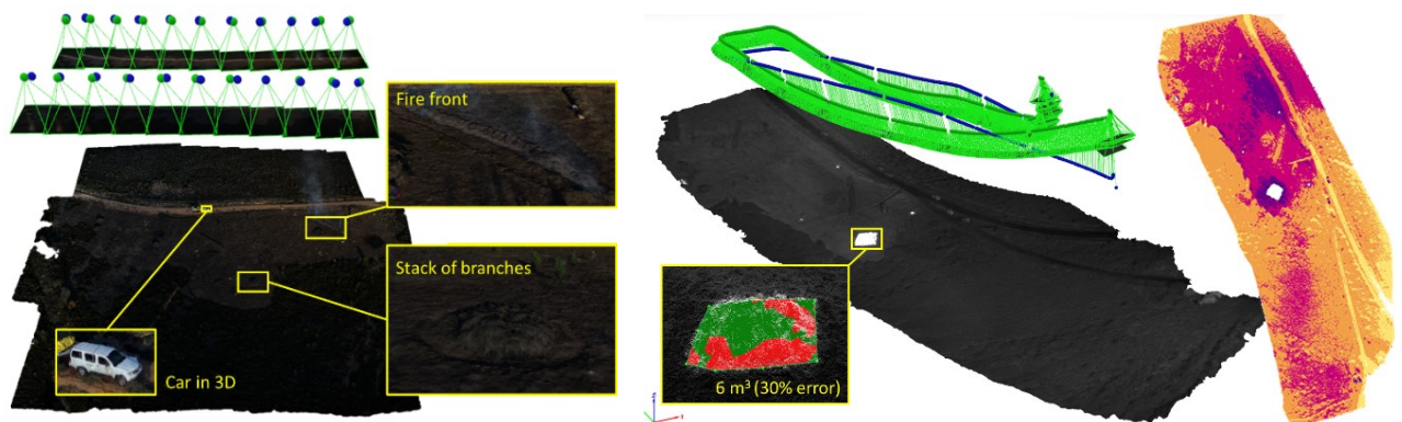
Fig. 6 Models of test area from UAV observation during test trials in Leon (November 2016): result from 200 visual HD-quality images (left) and when modelled from 2060 low-resolution (640x480) thermal images (right).
