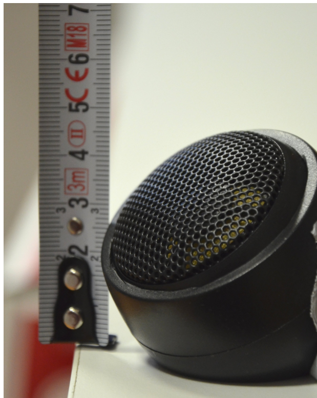
Figure 2. Determining the coordinates of loudspeakers with the ruler. Due to the hidden loudspeaker's membrane the positioning accuracy is estimated to 1 cm.
