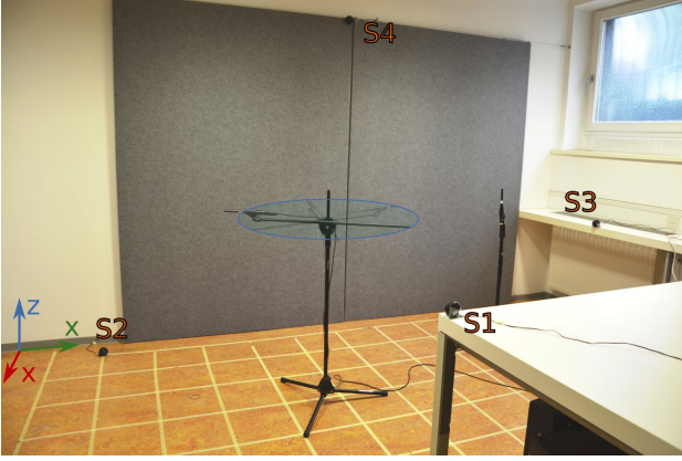
Figure 3. A photography of the room with the indication of the coordinate system (in the corner) the position of the four loudspeakers (S1, S2, S3 and S4) and the microphone stand with the boom arm that enabled the rotation of the microphone in a horizontal plain.
