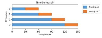
Fig. 4. Walk-forward Train-Test validation.
