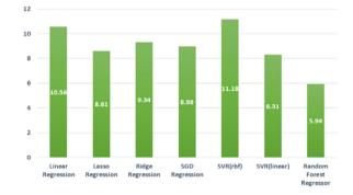
Fig. 16. 15 projects TD predictions – MAPE for 40 steps-ahead using Walk-forward Train–Test validation.
