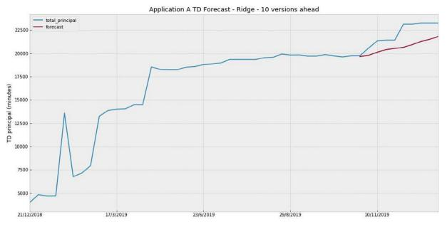
Fig. 19. Project A TD Principal forecasting for 10 steps ahead using Ridge (the ground truth from the starting point of the forecasts and onwards was hidden from the participants).
