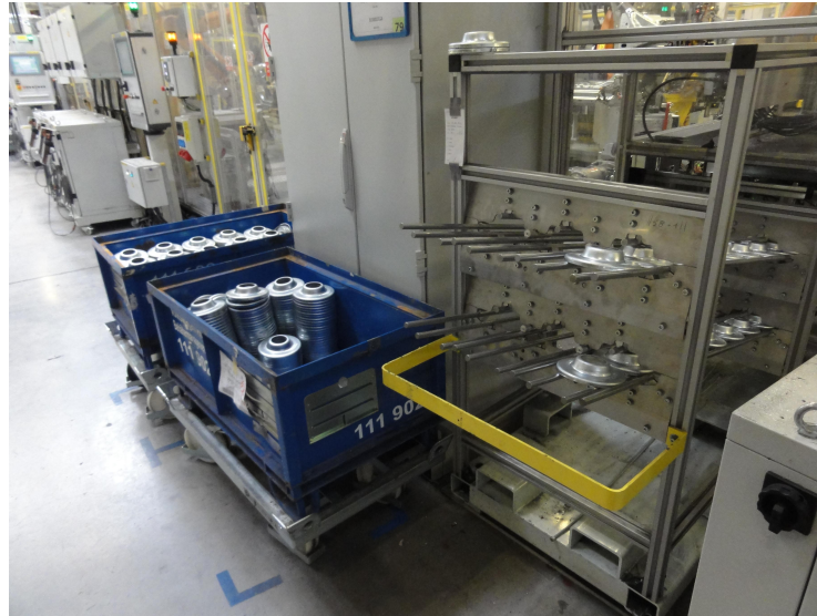
Fig. 1. Image of the transportation package with objects and feeder of the automatic assembly line
