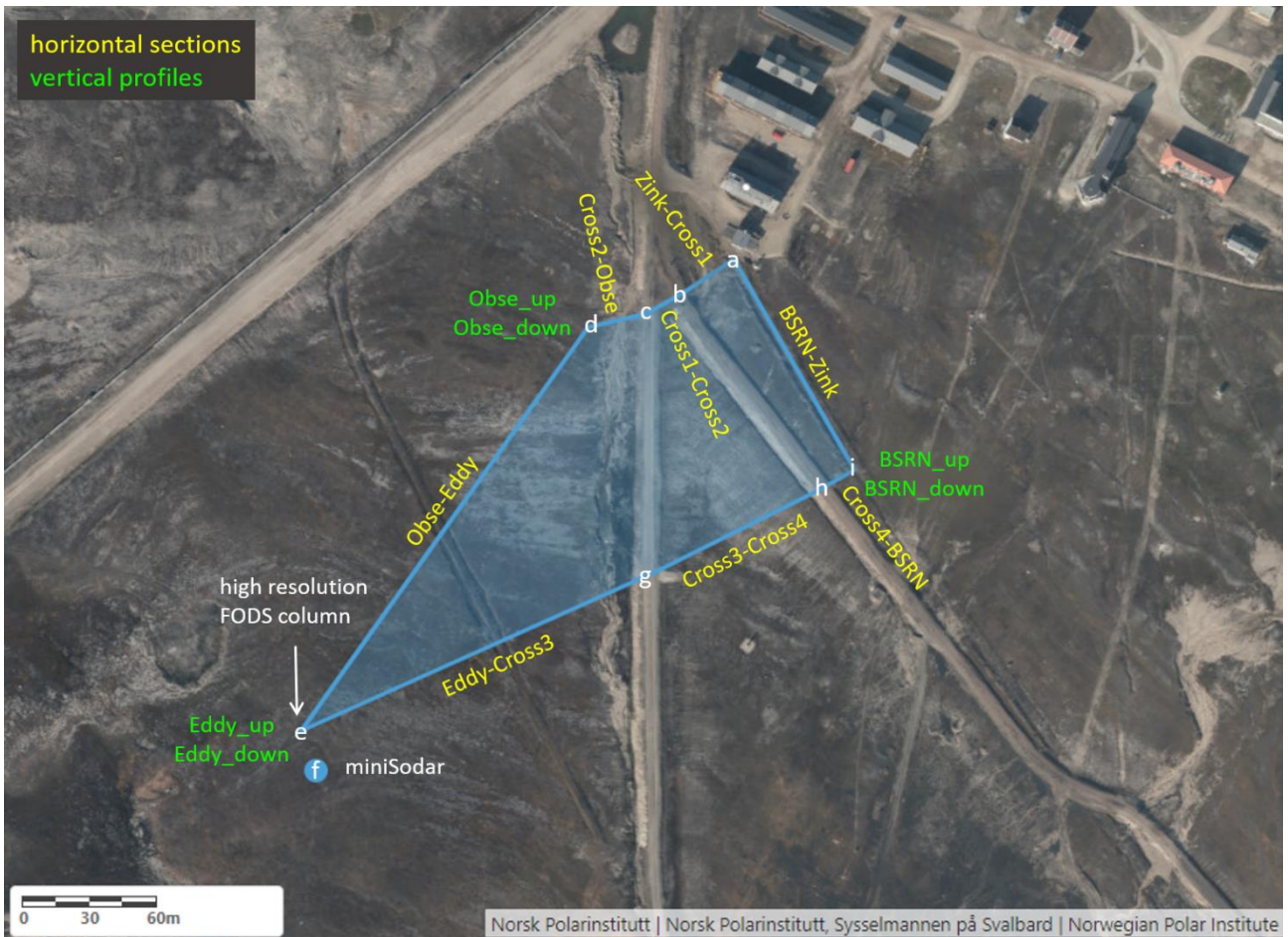
Figure 2. Setup south of Ny-Ålesund. The labels are the section names of the fiber optic Array (see File overview ). The letters a-i mark crucial points with their coordinates listed in table 1. The map source is Svalbardkartet ( geokart.npolar.no/Html5Viewer/index.html?viewer=Svalbardkartet ).
