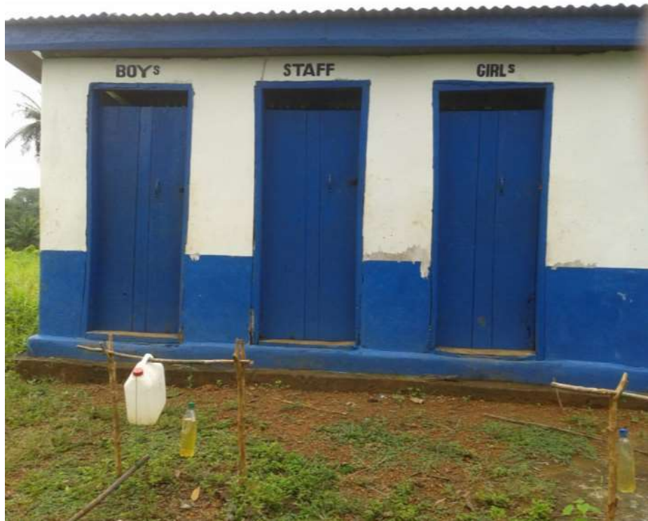
Tippy taps at a rural school in Sierra Leone. The tap is foot-operated, by applying pressure to the lever. The smaller bottle contains a disinfectant solution. Photo Credit: Rafael Mitchell
