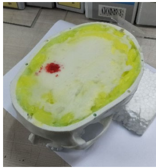
FIGURE 13: Head phantom with simulated stroke.
