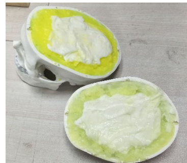
FIGURE 12: Head phantom without simulated stroke
