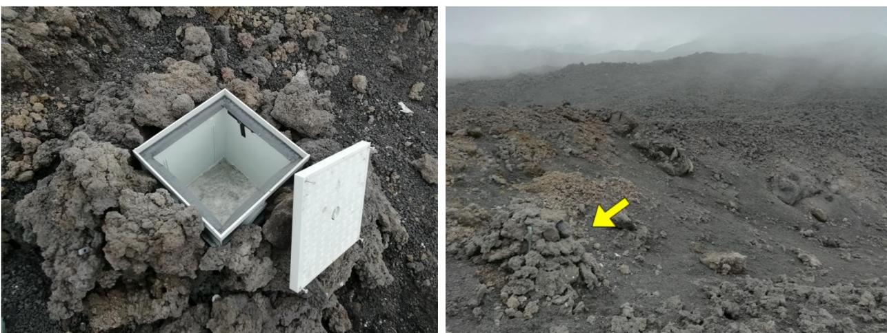
**Figure 15** – Left: on a check performed 28 days after its installation, the interior of the bottomless PVC box, installed on Etna at 2600m elevation, was dry, proving the reliability of the adopted sealing solutions. Right: the box at 2600m elevation is covered with ash and stones to make it less visible and to provide further protection against environmental factors.
