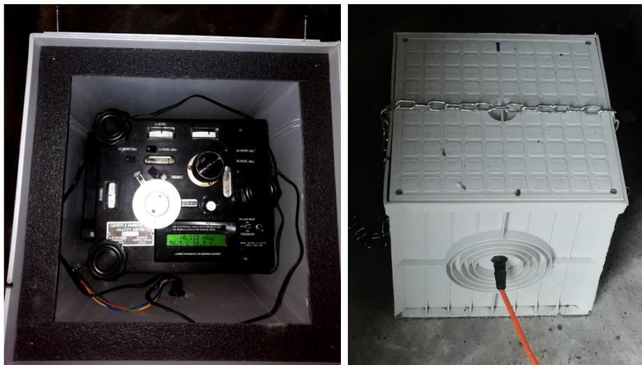
**Figure 11** – Left: L&R gravimeter inside the protective plastic box at the test installation site on Etna. Ambient temperature and atmospheric pressure sensors are visible on the left, inside the box (edge of the multicolor wire). Right: the protective plastic box is screwed onto the concrete base and sealed with silicon; it is closed with a lead firmly screwed onto sealing ribbon (visible as a black frame in the left panel).
