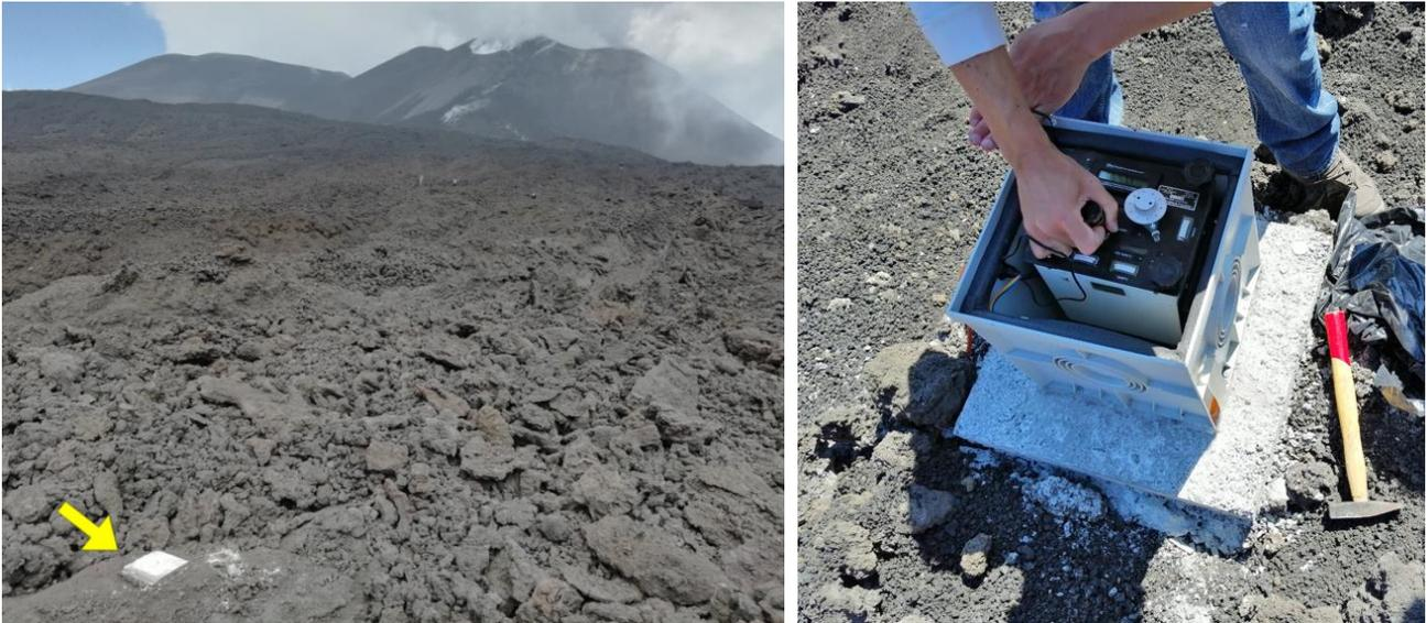
**Figure 14** – Left: concrete base on Etna at 2900m elevation. The summit active craters are visible in the background. Right: gravity measurements are performed with a L&R gravimeter on the concrete base at 2600m elevation.
