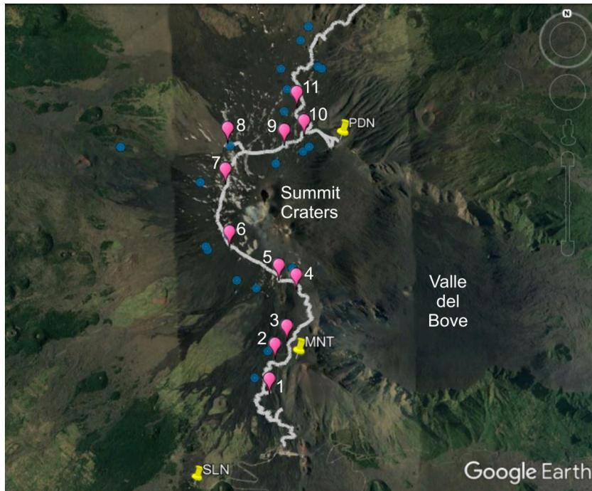
**Figure 5** - Preliminary optimal configuration of MEMS pixels (in blue) selected by the numerical algorithm of the GFZ team and sites identified as suitable for the installation of MEMS pixels during the field trip in June 2019 (purple symbols). Yellow pins mark the site where the two iGravs at higher elevations are installed (SLN and MNT) and the position of the Pizzi Deneri Observatory (PDN). Aerial photograph taken from Google Earth.
