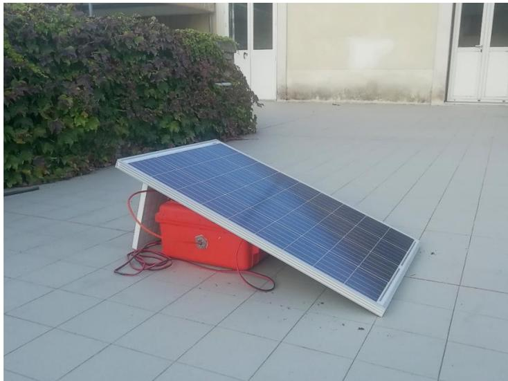
**Figure 7** – Setup of the test station installed in the facilities of INGV-OE between 6 and 21 August (see text for details). The solar panel on top of the orange case, containing most components of the station, are shown.
