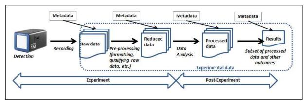
Figure 3: Simplified illustration of Classes of Experimental Data in the Science Life Cycle (from the Soleil Data Policy)
