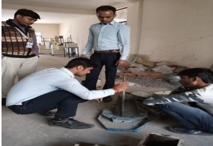
Fig.4:-Preparation of Slump test
