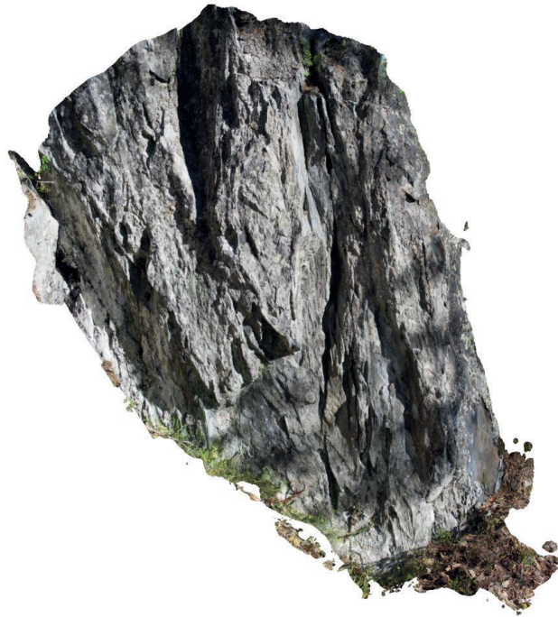
Figure 5: High-resolution, photogrammetric outcrop models generated using drones play a key role in the virtual course Applied Field Exploration generated in the EXpLORE project.
