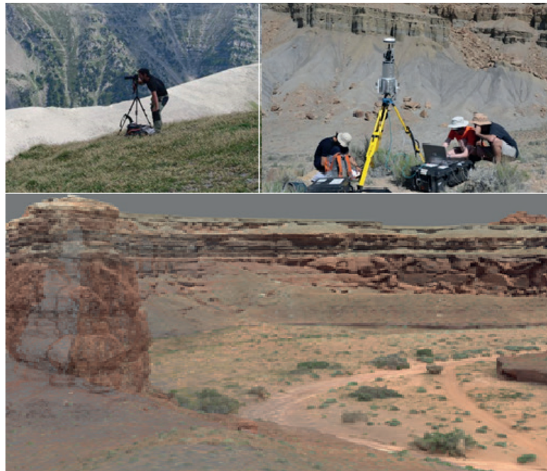
Figure 2: Common Digital Outcrop Modeling (DOM) techniques. Top left: convergent photogrammetry acquisition process. Top right: LIDAR acquisition device. Bottom: DOM of an eolian sandstone outcrop in Utah.
