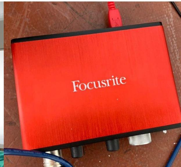
External sound card Focusrite Scarlett 2nd gen solo 44 100 Hz discretization
