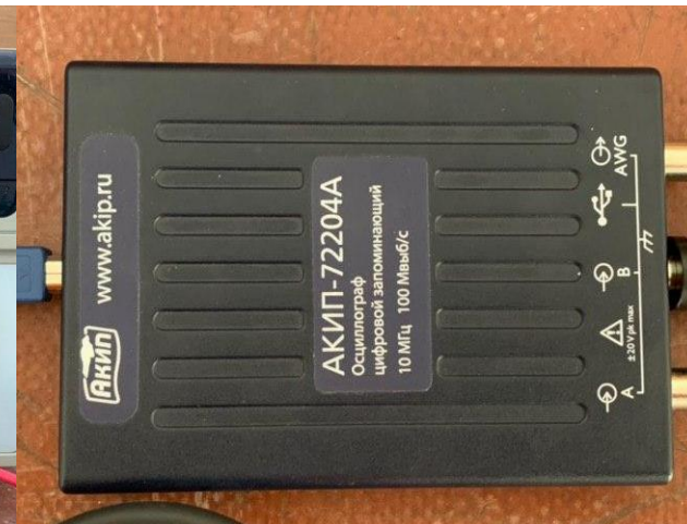
Digital oscilloscope AKIP-72204A Discretization up to 100 MHz
