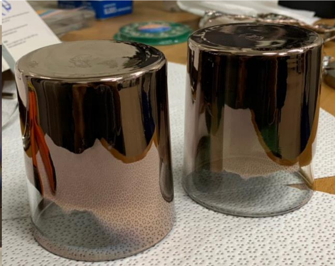
Sputtered glasses Aluminum 2\mu\text{m} \pm 30\text{nm}
