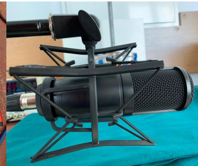
Condenser microphone AKG P120 (cardioid pattern) 20 Hz to 20 kHz response
