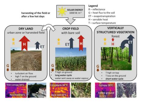
**Fig. 4.2** Solar energy distribution on different surfaces—dry land, crop field and forest. Thermal images show the surface temperature and thus provide information how the energy fluxes are distributed. Sensible heat (H) provides energy for fast ascending flux of air which transports humidity high into atmosphere. Water vapour released by vertically structured vegetation stays near the canopy and can return back in form of due or light rain
